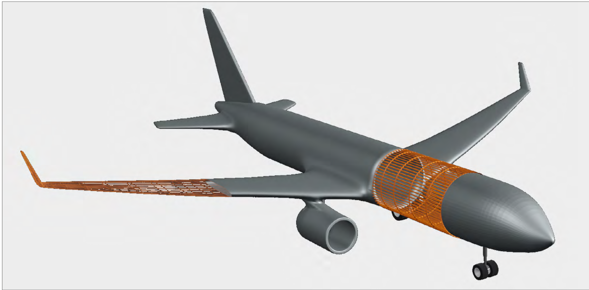
Figure 3.2: Schematic diagram of the airframe of a passenger aircraft, consisting of fuselage, wings, engine nacelle, cowling, tail and undercarriage (source: by kind permission of E. Tercero Daschner)
