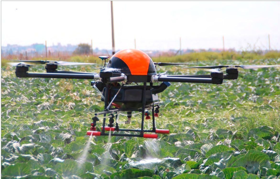
Figure 3.9: Unmanned 3D aircraft for application of plant protection agents
