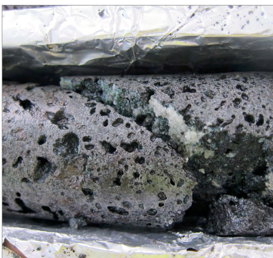
Figure 3.65: Permanent storage of CO 2 through mineralisation in a suitable geological deposit (source: Carbfix, photo by Sandra O. Snaebjornsdottir)
