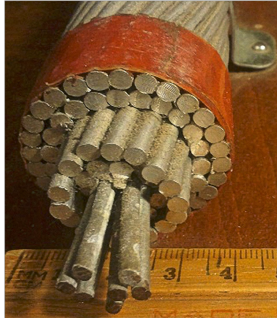
Figure 3.90: Steel-reinforced aluminium cable (source: Clark Mills, Sample cross-section of high tension power (pylon) line.jpg, CC BY-SA 3.0)
